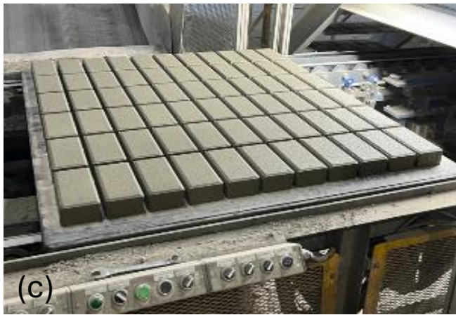
(a) Buckets of milled dry biochar right before mixing, (b) Funnel added to the plant mixer to add dry biochar; Freshly produced pavers with (c) CTRL_Paver and (d) 10% PYR-DOUG-FIR_Paver
