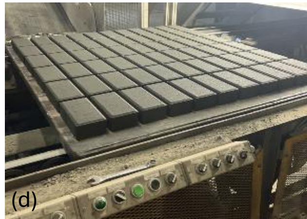
(a) Buckets of milled dry biochar right before mixing, (b) Funnel added to the plant mixer to add dry biochar; Freshly produced pavers with (c) CTRL_Paver and (d) 10% PYR-DOUG-FIR_Paver
